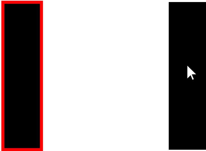
Figure 1: Fitts' Law Apparatus consisting of two clickable boxes. The red border around the box indicates the next box to be clicked.
